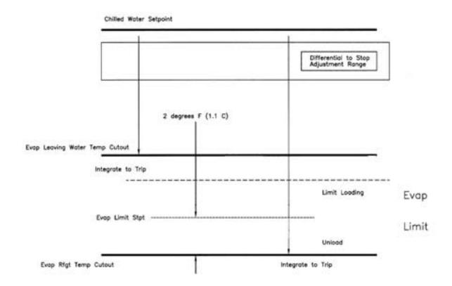
Limit Loading: The potential to limit loading increases as the saturated evaporator temperature approaches the evaporator limit setpoint.
